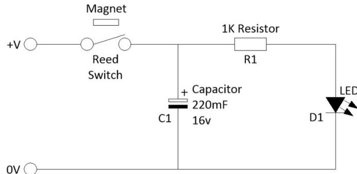
In the above circuit the capacitor is charged up when the Reed switch is closed, this also illuminated the LED. When the Reed switch opens the voltage stored in the capacitor will keep the LED illuminated until the capacitor is discharged.
