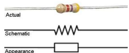
There are many different types and shapes of resistors but for the purpose you want a carbon film resistor is adequate. They are available in values from 1 Ohm to 10M Ohm, and different power rating (wattage)
