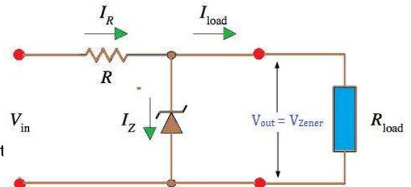
The Formula is Resistor Value( $R$ ) =  $(V_{in} - V_{out}) / I$  where  $I$  is the current required at the output.
